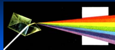
Refraction of white light by a prism
