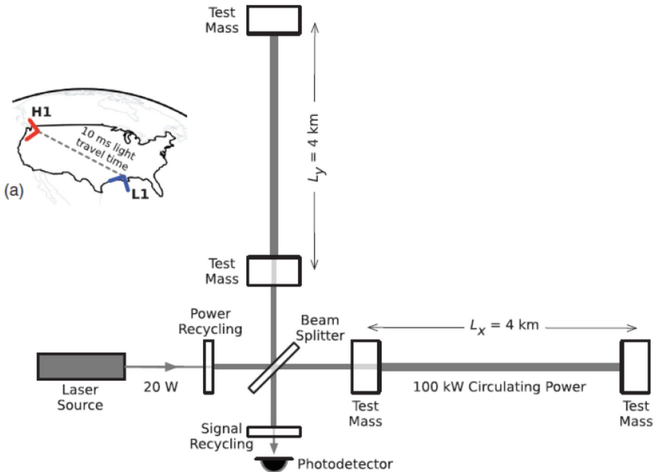
Fig 3: Diagram of a LIGO detector: Photons from a laser are fed into a set of 2 pairs of mirrors (the “test masses”) using a beam splitter. A passing gravitational wave will cause a ‘quadrupolar’ distortion of spacetime, so that if the path between one set of mirrors contracts, the other will lengthen, and vice-versa. This is measured by looking at interference between the 2 beams. The 2 detectors are separated by 3,000 km (light takes 10 milliseconds to travel this distance).
